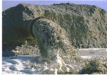
(b) Slurry and sediment transport in pipelines. Photograph courtesy of LI-Ceengineering [34].
